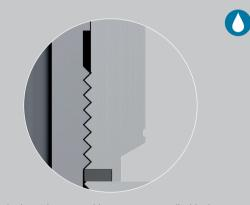
The lock nut has a marking groove on cylindrical Whitworth tube threads.
